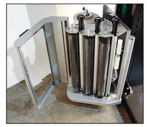
Patented triple knurled roller pre-stretch system with 225% powered pre-stretch. Easy thread design with safety door; if opened, shuts off machine.
